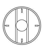
Installed with the shaft mounted vertically on the centre line of the vessel. Fitted with four strip baffles mounted vertically 90° apart with rotation clockwise when looking down the shaft so fluid is pushed down the vessel. This installation creates a turbulent fluid regime ideal for most mixing applications.
