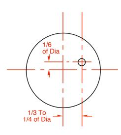
Installed with the shaft mounted vertically off centre without baffles with rotation clockwise when looking down the shaft so fluid is pushed down the vessel. The exact position depends upon the particular application and tank size. Provides good mixing without baffles. This technique places the propeller in a position which provides an acceptable flow pattern but inferior to a fully baffled tank.
