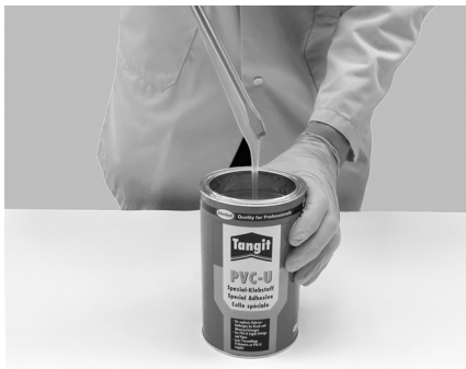
Checking the cement
