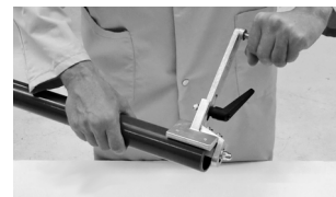
Chamfering the pipe
