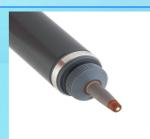
The membraned amperometric chlorine sensors, are enhanced with a third, reference electrode which eliminates zero drift. Its unique design means that pH correction is not usually required at all, completely eliminating reagents.
