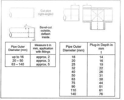
Preparation of the surfaces to be bonded:
