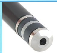
The membraned amperometric chlorine dioxide sensor is a two electrode sensor which operates at an elevated applied potential which in turn eliminates zero drift. It's unique design means no reagents or buffers are required at all and calibration is a simple one point (no zero required) operation.
